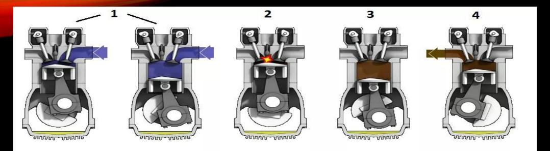
In these engines, the combustion of a fuel releases a high-temperature gas, which, as it expands, applies a force to a piston, moving it. Thus, combustion engines convert chemical energy into mechanical work. Decades of engineering by many scientists went in to designing the internal combustion engine, which took its (essentially) modern form in the latter half of the 19th century.
